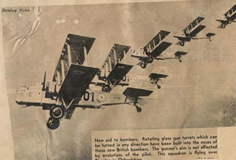
New aid to bombers. Rotating glass gun turrets which can be turned in any direction have been built into the noses of these new British bombers. The gunner's aim is not affected by evolution of the pilot. This squadron is flying over Gloucester in Oxfordshire.
