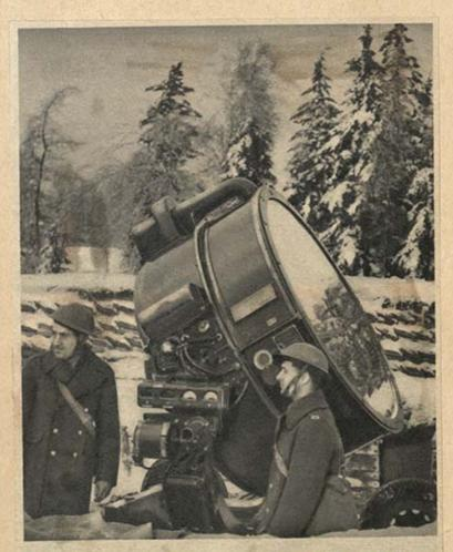
**EIGHT HUNDRED MILLION** candle-power searchlights such as the one above are also linked with the anti-aircraft units. On a clear night, such searchlights can penetrate 30,000 feet and each has its own self-contained power plant. Crews are linked to headquarters by telephone
