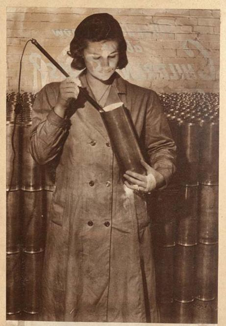
THE LONG test lamp is like a magic wand. Joan uses it to check the interior of shell case. If it is O.K. it goes into "stock" and the famous broad arrow of the British Government is punched into its bottom with a ringing noise like a chime
