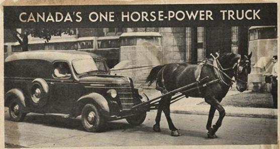
"THE HORSELESS CARRIAGE" gets a horse in this picture from Montreal. A baker there figured he had better get ready for more extensive gasoline rationing so he removed the engine, transmission and drive shaft from a truck, put dobbin out front and ran a pair of reins under the windshield.
